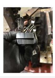
14. Brush Holder Condition - Verify proper gap to Commutator
