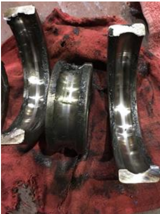
Frosted and grease contamination
