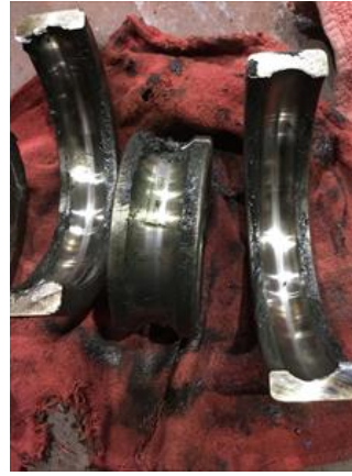
Frosted and contaminated grease
