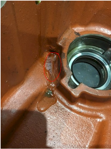
Water in remaining oil and metal shavings
