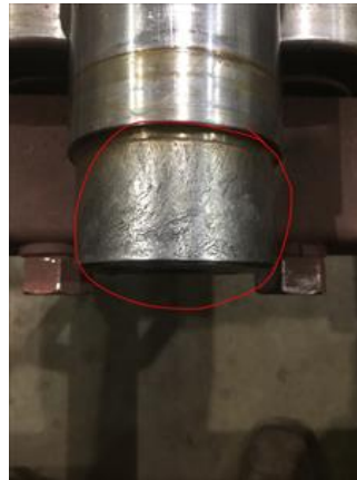
Excessive wear where the gear rides
