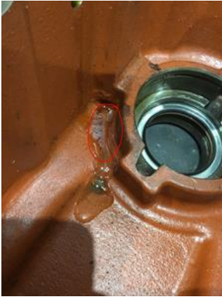
Water in remaining oil and metal shavings
