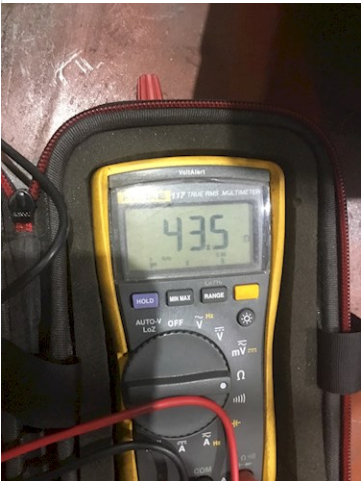
21. MegOhms between Fields and Series
