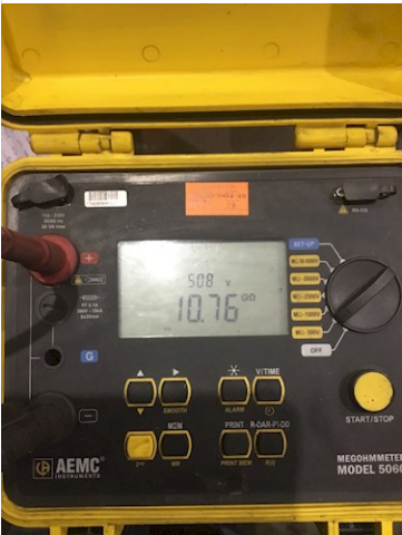
21. MegOhms between Fields and Series
