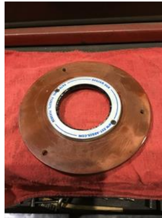
Installed Agis ring on D.E. Bearing cap
