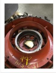
61. Opposite Drive End - Endbell Bearing Fit Condition (P) Pass 62. Bearing Cap Condition Drive End Bearing Cap Opposite Drive End Bearing Cap **Pass Pass** 63. End Bell Air Seal Fits Drive End Air Seal Opposite Drive End Air Seal **Pass Pass** 64. List Machine Work Needed Below Repair drive end shaft bearing fit. Normal turn and metalizing. 65. Technician **Brandon Woodard**
