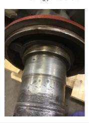
54. Drive End Bearing Shaft Fit Condition
