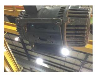
4. Describe the Overall Condition of the Equipment as Received Electrical good. Bearing failure.
