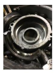
Drive End - Endbell Bearing Fit Condition (P) Pass
