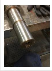
54. Drive End Bearing Shaft Fit P54
