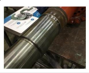
56. Drive End Bearing Shaft Fit Condition
