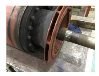
58. Opposite Drive End Bearing Shaft Fit Condition
