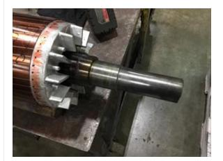
54. Drive End Bearing Shaft Fit Condition
