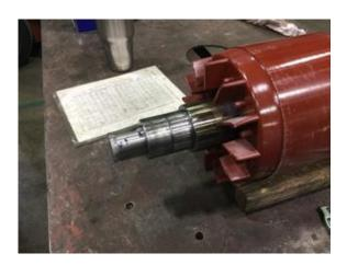
57. Opposite Drive End Bearing Shaft Fit Condition
