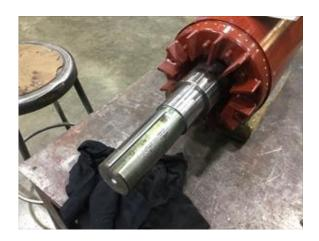
55. Drive End Bearing Shaft Fit Condition
