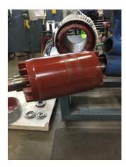
48. List the Parts needed for the Repair Below (2) 6312 bearings
