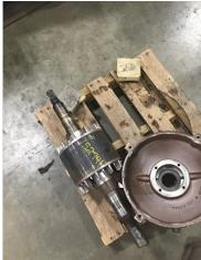
48. List the Parts needed for the Repair Below 6210 2RSC3 bearing 62092RSC3 bearing
