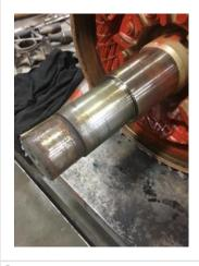
56. Opposite Drive End Bearing Shaft Fit Condition
