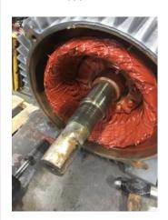
54. Drive End Bearing Shaft Fit Condition
