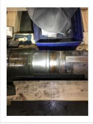
54. Drive End Bearing Shaft Fit Condition
