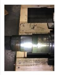
Opposite Drive End Bearing Shaft Fit Condition (P) Pass
