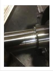
56. Opposite Drive End Bearing Shaft Fit Condition (P) Pass
