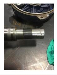
52. Coupling Fit Closest to the end of the Shaft
