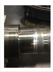
54. Drive End Bearing Shaft Fit Condition
