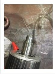
68. Opposite Drive End Bearing Shaft Fit Condition
