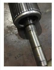
66. Drive End Bearing Shaft Fit Condition
