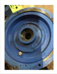
71. Drive End - Endbell Bearing Fit Condition (P) Pass
