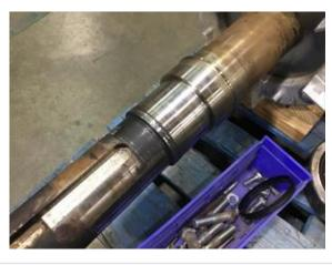
54. Drive End Bearing Shaft Fit Condition
