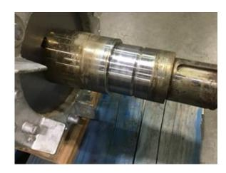
Opposite Drive End Bearing Shaft Fit Condition
