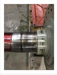
58. Opposite Drive End Bearing Shaft Fit Condition
