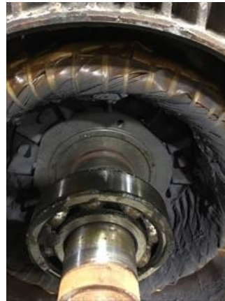
Bearing cap bolts missing on ODE.
