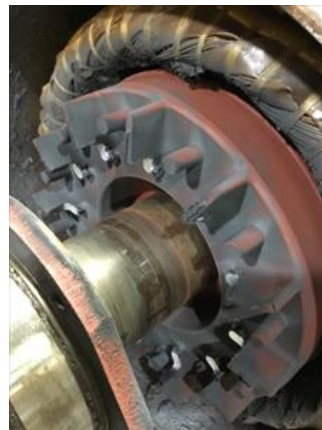
Bearing cap bolts missing on ODE.
