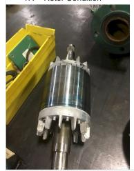
48. List the Parts needed for the Repair Below 6206 C3 6205 C3 Mechanical seal
