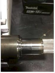
57. Opposite Drive End Bearing Shaft Fit Condition
