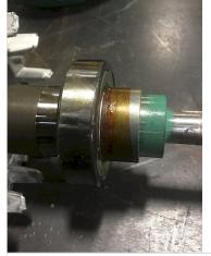
P33 Drive End Bearing Condition **Normal Wear**
