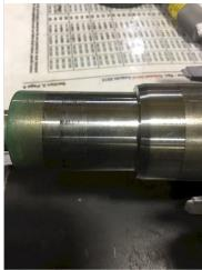
55. Drive End Bearing Shaft Fit Condition
