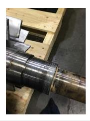
Drive End Bearing Shaft Fit Condition (P) Pass 54. Opposite Drive End Bearing Shaft Fit
