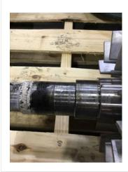
56. Opposite Drive End Bearing Shaft Fit Condition (P) Pass
