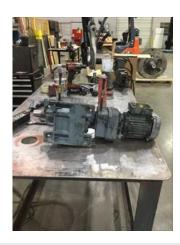
Describe the Overall Condition of the Equipment as Received Rewind needs new fan no machine work
