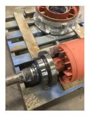
32. Drive End Bearing Condition Normal wear P82
