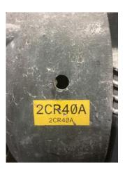
ODE grease fitting not lined up.
