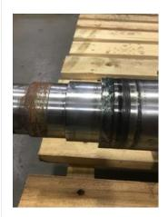
Opposite Drive End Bearing Shaft Fit Condition (P) Pass
