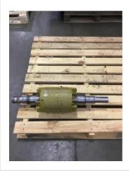
47. List the Parts needed for the Repair Below Rewind 6312 C3 x2
