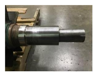
56. Drive End Bearing Shaft Fit Condition
