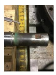
53. Drive End Bearing Shaft Fit
