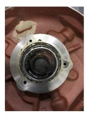
30. Drive End Bearing Insulation or Grounding Device? none present
