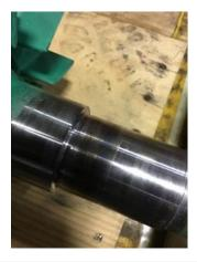
54. Drive End Bearing Shaft Fit Condition
