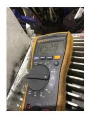
26. Stator Overloads/Ohms
