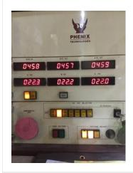
84. Test Run Amperage
