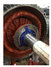
80. Final Insulation Resistance Test
