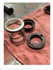
81. DE Seal Type/Size mechanical carbon / sic
