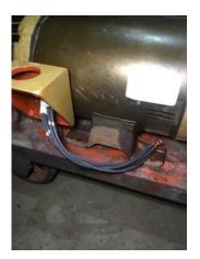
88. Final Insulation Resistance Test 171.9 Gigohms P31
