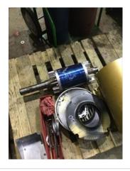
48. List the Parts needed for the Repair Below 1-6312 Bearing 1-6309 Bearing
