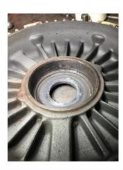
60. Drive End - Endbell Bearing Fit Condition(F) Fail
