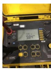
77. Final Insulation Resistance Test
