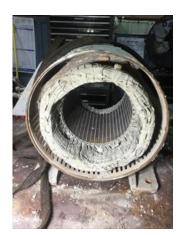
4. Describe the Overall Condition of the Equipment as Received Covered with concrete.
