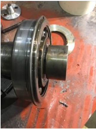
Bearing is off the shoulder.
