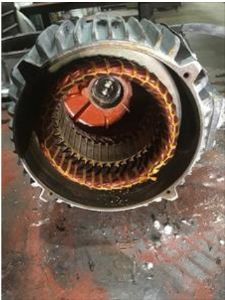
Bearing is off the shoulder.
