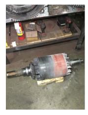
**Growler Test** (Pass) Pass 44. 45. Number of Rotor Bars 71 46.
