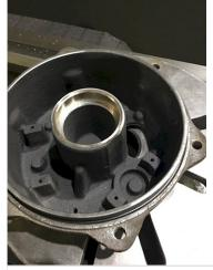
102. Bearing Cap Condition Post Repair
