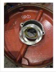
40. Opposite Drive End Bearing Condition cage failure P118
