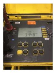
18. Interpole Circuit Insulation Resistance to Ground
