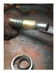
Assembled Shaft Runout 0.002 Inches
