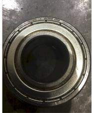
Opposite Drive End Bearing Number-34. 6205 35. Opposite Drive End Bearing Qty. 36. Opposite Drive End Bearing Type (Ball) Ball Bearing 37. Opposite Drive End Lubrication Type (Grease) Grease Lubricated Opposite Drive End Bearing Insulation or Grounding Device? 38. P99 Opposite Drive End Wavy Washer/Snap-Ring Other Retention Device? 39. wavy washer
