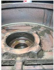
60. Opposite Drive End - End Bell Bearing Fit 0 Degrees 60 Degrees 120 Degrees 3.5436 3.5434 3.5435 61. Opposite Drive End - Endbell Bearing Fit Condition (NA) Not Applicable 62. Bearing Cap Condition Drive End Opposite Drive End 63. End Bell Air Seal Fits Drive End Air Seal Opposite Drive End Air Seal List any Machine work Needed Below D.E housing fit bad Signature of Technician Performing Measurements **Terrence Holland**
