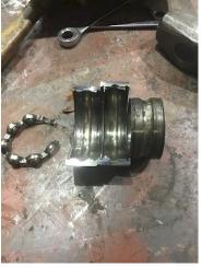
Caused by grease contamination.
