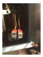
14. Brush Holder Condition - Verify proper gap to Commutator
