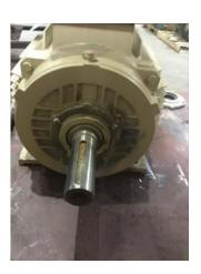
7. Assembled Shaft Runout 0.002 Inches 8. Assembled Shaft End Play inches 9. Air Gap Variation <10%
