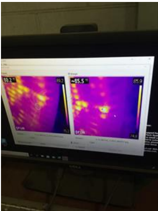
After hottest spot had a 10 degree rise after 2 minutes
