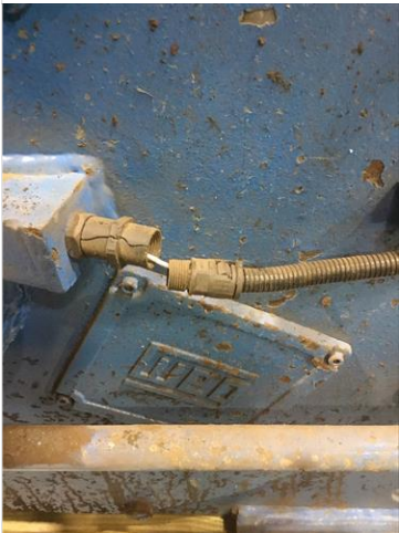
Drive end RTD plastic cracked
