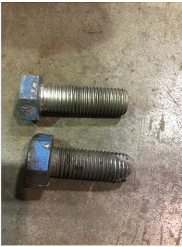
Correct metric bolt on top, wrong standard bold on bottom.
