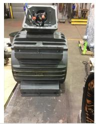
Describe the Overall Condition of the Equipment as Received Burned up stator
