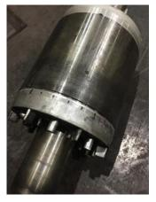
D.E bearing suffered total cage failure due to lack of lubricant. This caused to rotor to drop onto the stator core and short out the windings.
