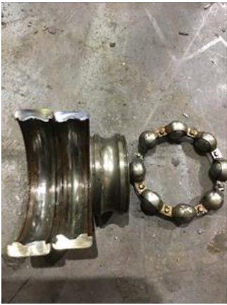
Damage due to contaminated lubricant
