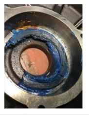
65. Root cause of failure Moisture contaminated grease.
